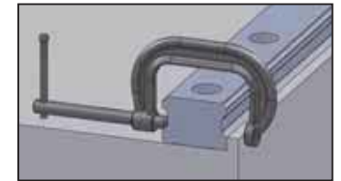
Fig 1.11.13 Mounting the master Linear Guide rail
